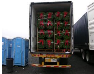
Rack 96 — build on pallet, each side has 8 posts, 6 pieces per post.
